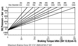
Maximum Braking Force SH 12.9: 30kN (6744.27 lbf) Minimum Pressure for full retraction: 100 bar (1450 psi) Weight of caliper and thruster - 52kg (114.64 lb) Weight of thruster only - 18kg (39.68 lb) Volume displacement of thruster at full retraction = 56ml (1.89 fl oz)
