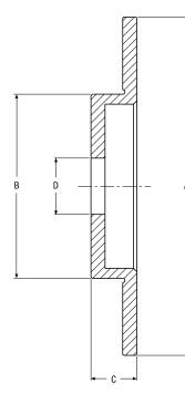
Twiflex brake discs may be supplied bored and drilled to customer requirements. Non-standard disc sizes, not shown in the tables, can be supplied to order. Brake discs are manufactured
