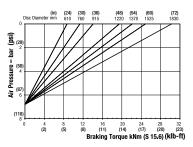
Maximum Braking Force S 15.6: 36kN (8093.12 lbf) Minimum Pressure for full retraction: 8.4 bar (122 psi) Weight of caliper and thruster - 49kg (108.03 lb) Weight of thruster only - 15kg (33.07 lb) Volume displacement of thruster at full retraction = 1.31ml (0.04 fl oz)
