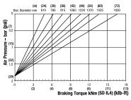
Maximum Braking Force SD 8.4: 19.5kN (4383.77 lbf) Minimum Pressure for full retraction: 2.4 bar (35 psi) Weight of caliper and thruster - 52.2kg (115.08 lb) Weight of thruster only - 18.2kg (40.12 lb) Volume displacement of thruster at full retraction = 2.51ml (0.08 fl oz)
