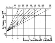
Maximum Braking Force SD 15.6: 36kN (8093.12 lbf) Minimum Pressure for full retraction: 4.6 bar (67 psi) Weight of caliper and thruster - 55kg (121.25 lb) Weight of thruster only - 21kg (46.29 lb) Volume displacement of thruster at full retraction = 2.51ml (0.08 fl oz)
