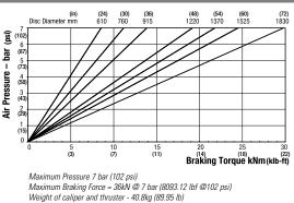
Weight of caliper and thruster - 40.8kg (89.95 lb) Weight of thruster only - 6.8kg (14.99 lb) Volume displacement of thruster at full stroke = 1.8 ml (0.06 fl oz)
